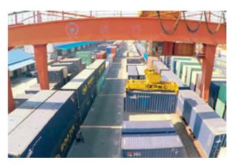
Transfer of containers between 1435 mm standard gauge and 1520 mm broad gauge rolling stock on the China-Russia border.
