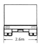
Note: Side cargo overhangs from the two sides of the vehicle cannot exceed 30cm.
